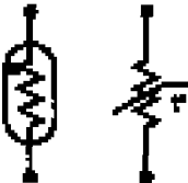
Figure 3.32. Symbols commonly used to represent a thermistor.
