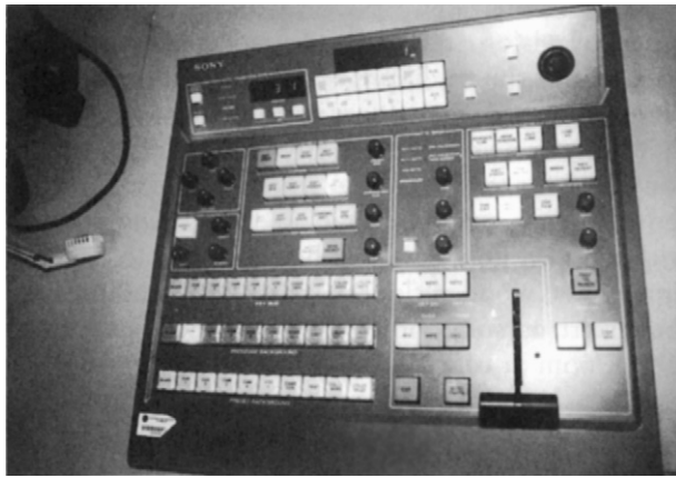
Figure 2.3 A close up of the switcher in the control room in Figure 2.2a. Although small, it can super, wipe, key graphics, and handle limited chroma key productions.
