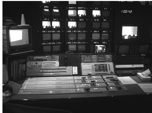
Figure 2.4 A larger production switcher. This switcher can perform all of the functions performed by the switcher in Figure 2.3, and can also affect, dissolve, or wipe from one level to the next. Larger switchers are capable of a greater number of effects. Some switchers are designed for editing and may be similar in appearance.
