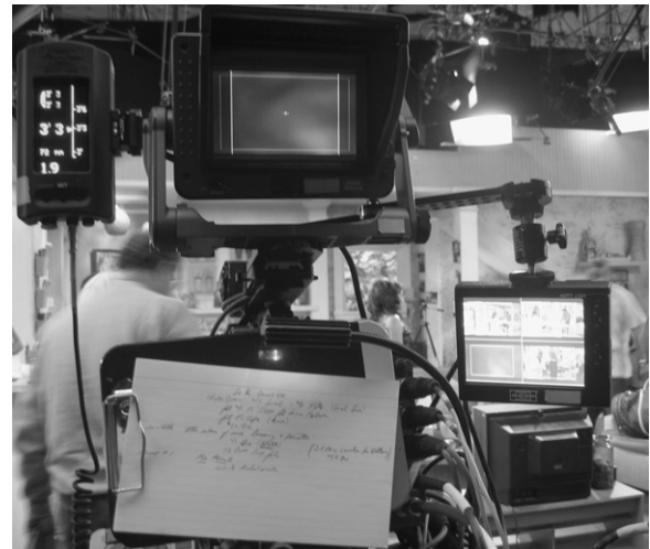
Figure 6.20 A cameraperson’s working view of a set using the quad split method. In the upper left is a “smart lens” reader that lets the camera operator know where the camera is focused and the depth field at that point. To the right of that is the viewfinder, marked for 4/3 and 16/9 formats. Under the viewfinder is a holder for the shot sheet. Hanging off to the right is a quad split screen that shows what each camera is shooting.
