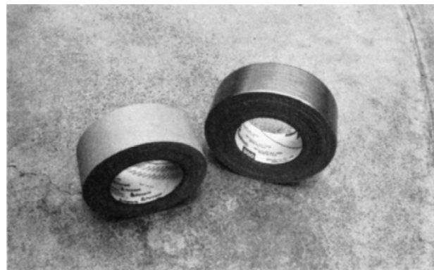
Figure 2.5 On the left is gaffer tape, which is strong and bears weight well. It is dull gray, so it is nonreflective, and it can be removed without leaving a residue. Duct tape, on the right, costs about a third or less, but it reflects light and often leaves a residue when removed.
