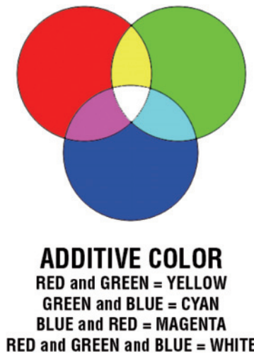
Figure 6.6: The additive mix system for generating color as used in electronic display devices such as cathode ray tubes.
