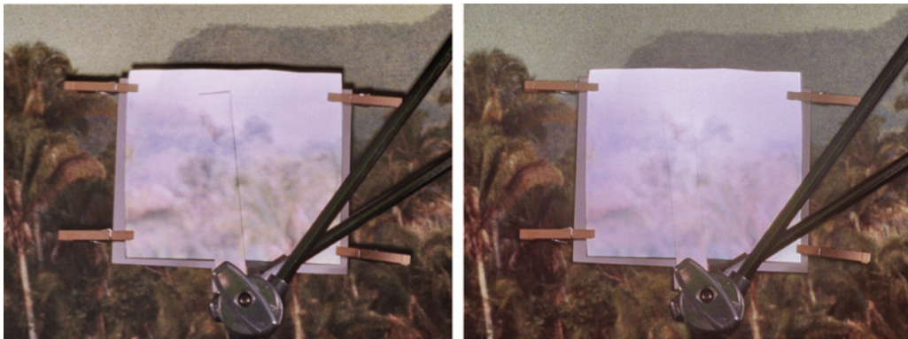
Figure 12.8: If you have to align your own optics, one trick is to place a small strip of Scotchlite in front of the screen to see whether it hides its own shadow. If the optics are misaligned, then a shadow edge will be clearly apparent, as in the picture at the left. To align the optics, gently move the camera over to the side or up and down as necessary until the shadow disappears, as in the picture on the right. The brighter foreground screen is the virtual background product and the dimmer screen behind is the Reflecmedia screen. Though both can be used for front projection, the virtual background material is a better choice for this application.
