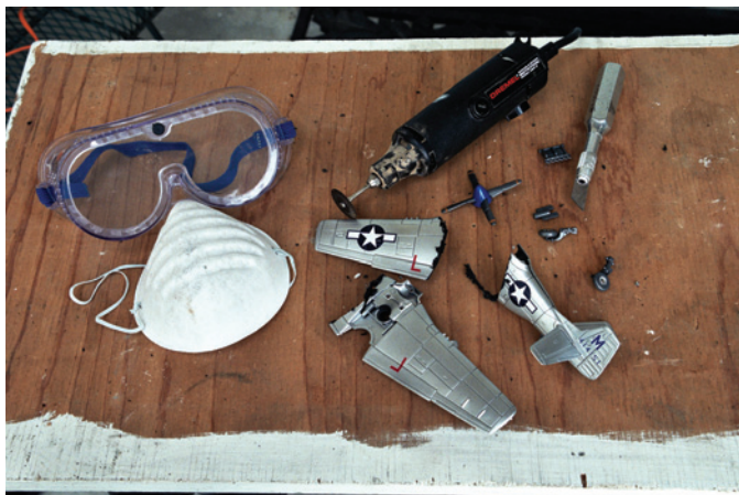
Figure 1.12: The model can be cut with a Dremel tool, hacksaw, or utility blade. Be sure to wear protective gear!
