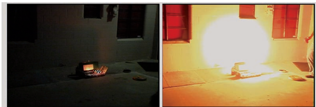
Figure 11.5: The pre-explosion photo on the left used only ambient light with the gain control of the camera set to the highest setting. This allowed the set to be seen, but it placed the flame so far above peak white that when the explosion went off in the photo at the right there is absolutely no detail and the fireball goes into clip instantly.
