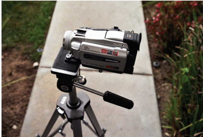
Figure 1.16: My camera is bolted so that it can slide forward and backward in the slot toward and away from the center of rotation of the tripod. The camera was positioned so that the center of the lens is atop the pivot point of the tripod. This is a good starting position for finding the nodal point.
