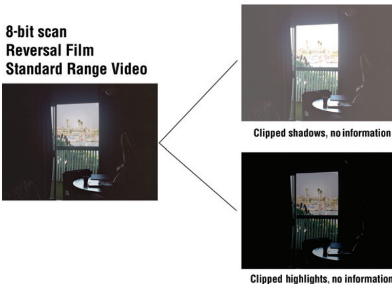
Figure 6.3: An 8-bit linear scan, while looking acceptable at one setting, such as reversal film or video, does not have a wide range for adjustment. If the file is brightened, there is no information in the dark interior, and if the file is darkened, the bright sky will go dull.
