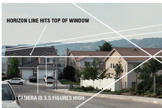
Figure 2.13: Finding the reference point for the horizon and getting a rough estimate of camera height. The actress was approximately 5.5 feet tall; if she was stacked on top of herself until her stacked figures reached the horizon and the figures were counted, it could be seen that the camera was located 5.5 feet/figure \times 3.5 figures = 19.25 feet above the point where the actress was standing.
