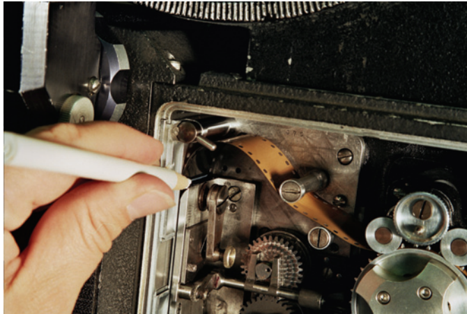
Figure 2.9: Marking the frame line.
