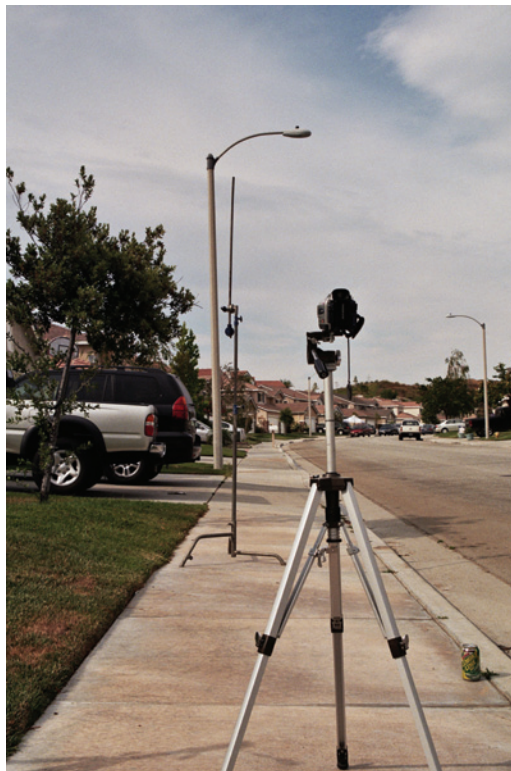
Figure 1.17: A setup for adjusting to nodal point. To find the nodal point, position a vertical pipe close to the camera almost in alignment with a light pole in the distance. Set the zoom to the widest focal length. Pan the camera and take note of the gap between the poles. If the gap opens and closes as you pan, you are not on nodal.
