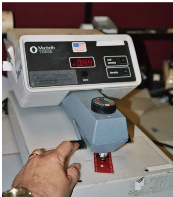
Figure 5.3: A densitometer reads the density of film, or how opaque it is to light. For color film, the wheel above the sensor can select a red, green, blue, or clear filter to get different color readings off the film. The number display indicates that the film being read has a density of 0.44 to white light.
