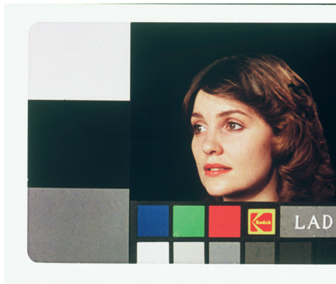
Figure 5.25: A Kodak girl head control. The gray box in the lower left hand corner should read red 1.00, green 1.45, and blue 1.55 on the internegative of this image. The readings are taken on a densitometer. Keeping gray as a pure gray is a system that holds over into the digital age.
