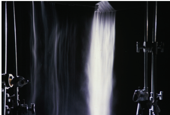
Figure 2.21: Falling baking soda powder shot at high speed was often used for waterfall elements. A power drill with a bent center bit in the chuck provided the vibration to set the powder going. The camera is in the foreground, wrapped in protective plastic. The powder is falling just in front of the camera. Featured are Lynn Ledgerwood and operator Adam Kowalski. Courtesy of Illusion Arts.
