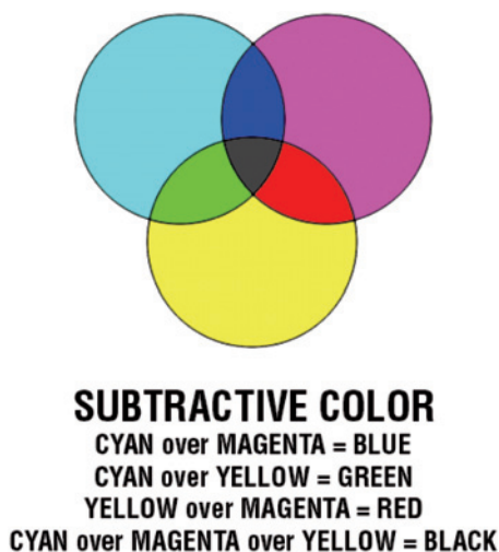
Figure 5.12: Subtractive color reproduction. When the secondary color dyes overlap, they reproduce the primary colors of red, green, and blue. The combinations of various densities of the cyan, magenta, and yellow dye can produce an enormous range of colors.
