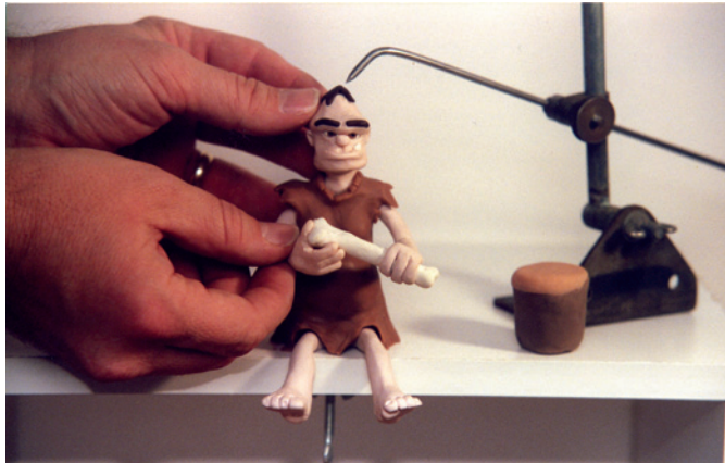
Figure 3.5: A typical stop motion animation setup. Out of view of the taking camera, the figure is “tied down” by being bolted to the table from underneath. The device to the right is a surface gauge. This gauge is used as a reference pointer to show the animator the previous position of the puppet when it is manipulated for the next frame. After the puppet is positioned, the gauge is removed and the frame is exposed. Digital capture systems such as the Stop Motion Pro product allow the previous frame to be superimposed upon the current frame on a video monitor to create an ultra precise reference of the puppet’s location on the previous frame. From How to Create and Animate a Clay Puppet , available from www.firstlightvideo.com .
