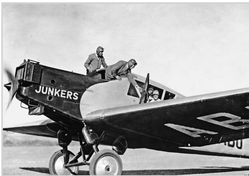
Entering service right after World War I, the Junkers F 13 seated four passengers in a plush, fully enclosed cabin.
