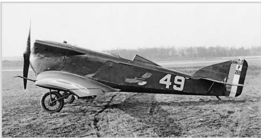
The Verville-Sperry R-3 racer of 1922 marked the U.S. emergence of an advanced configuration pioneered by Germany's Hugo Junkers.
