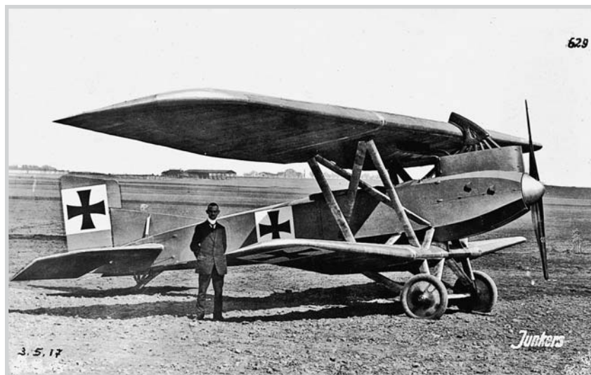
Designed for strafing trenches, the armored Junkers J 4 of 1917 was history's first production airplane made entirely of metal.
