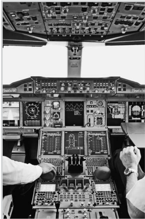
Modern jetliners like the Airbus A380 rely on computerized “glass cockpits,” so named for their instrument display screens.
