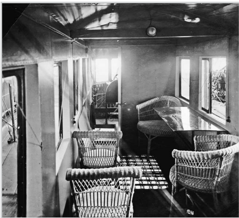
Equipped with wicker chairs, picture windows, a writing table, and electric lights, the first Ilya Muromets drew obvious inspiration from luxury rail travel. The door to the airplane's dual-controlled cockpit stands open.
