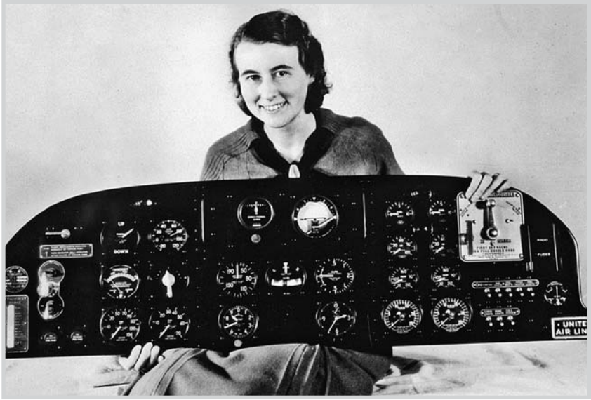
The center of the Boeing 247 instrument panel had three gyro instruments for blind flying: a directional gyro (top left), artificial horizon (top right), and turn-and-bank indicator (middle).
