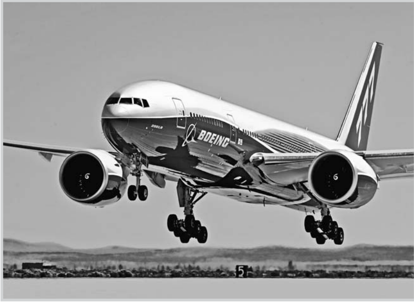
The Boeing 777, the world's largest twin-engine airplane, has enormous fanjet engines that produce up to 115,000 pounds of thrust each.
