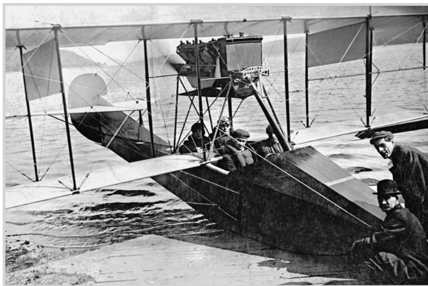
The Curtiss F-Boat of 1912 was history's first boat-hulled airplane.
