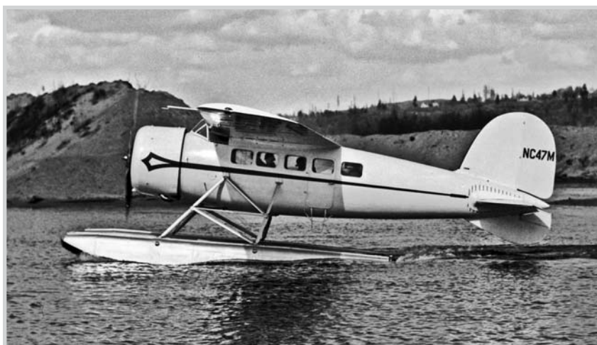
The Lockheed Vega set numerous speed and distance records at the hands of Amelia Earhart, Wiley Post, and other noted aviators. Introduced in 1927, the Vega combined cantilevered wings with a semi-monocoque fuselage of molded plywood.
