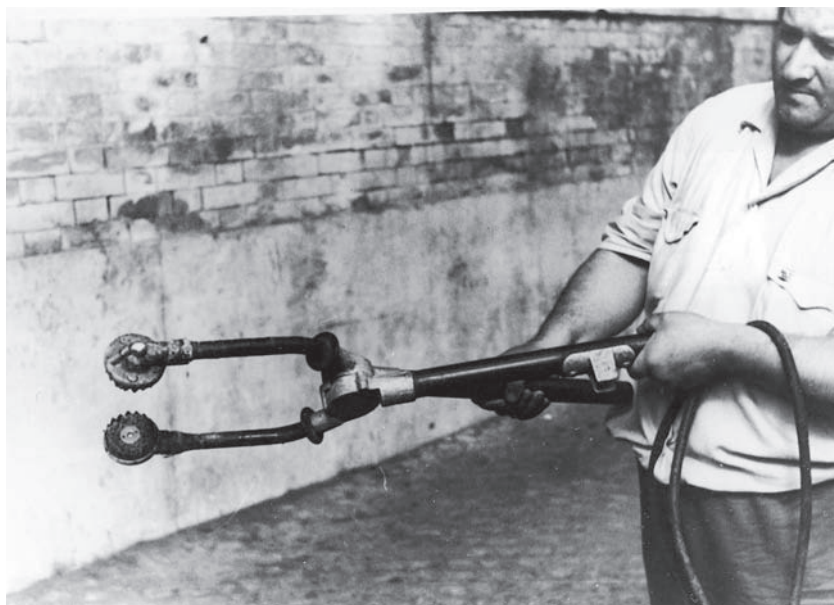
Electrodes used in the Rome municipal slaughterhouse to stun pigs, c. 1938. Sapere , no. 154 (May 1941).
