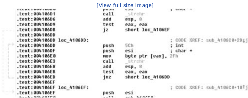
Figure 6-10. The code here is using an API call strchr to find character 5Ch (\) in a string. Once the character is found, the code uses mov byte ptr [eax], 2Fh to replace the back slash with character 2Fh (/) . This loops until no more back slashes are found (via the test eax, eax and subsequent jnz , which jumps [if not zero] back to the beginning of the loop).
