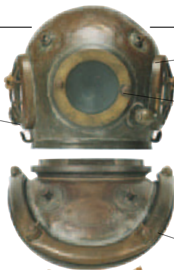
Helmet equipped with two-way communication system so diver can talk to someone on the surface
