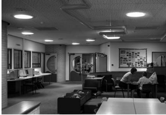
Intelligent use of light pipes can slash lighting costs (Courtesy of Monodraught)
