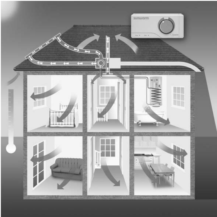
The Sunwarm system uses solar heated air for space heating and DHW (Reproduced with permission from Nuaire)
